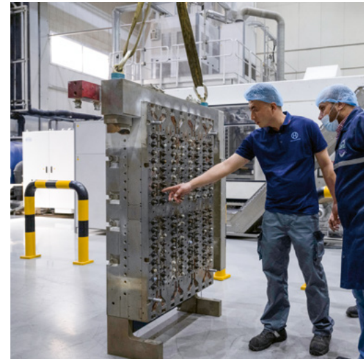
Hot runner M144-011 is uncrated and inspected for any transport damage during cleaning.
