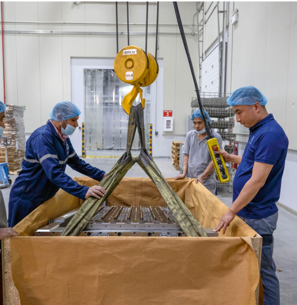
Hot runner M144-011 is uncrated and inspected for any transport damage during cleaning.
